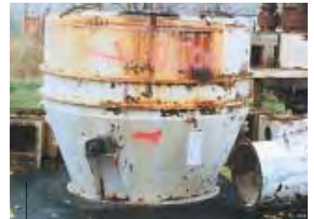
Classifier Housing before Refurbishing
