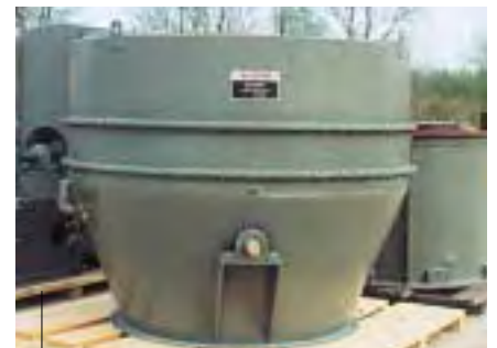
Refurbished Classifier Housing
