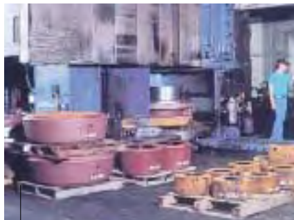
Pulverizer rolls being machined
